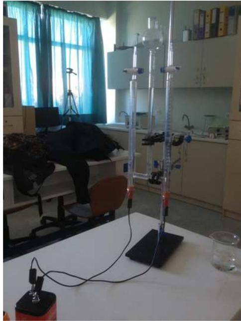
**Figure 1: The Electrolysis Apparatus**
