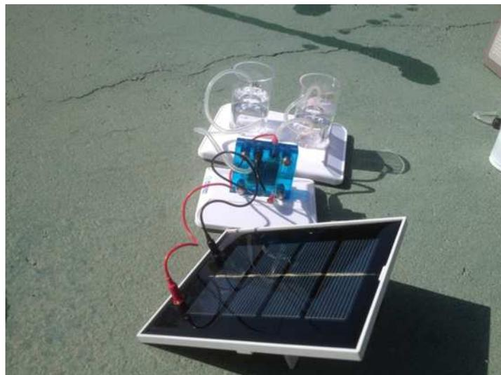
**Figure 2: Water Splitting using Solar Energy**
