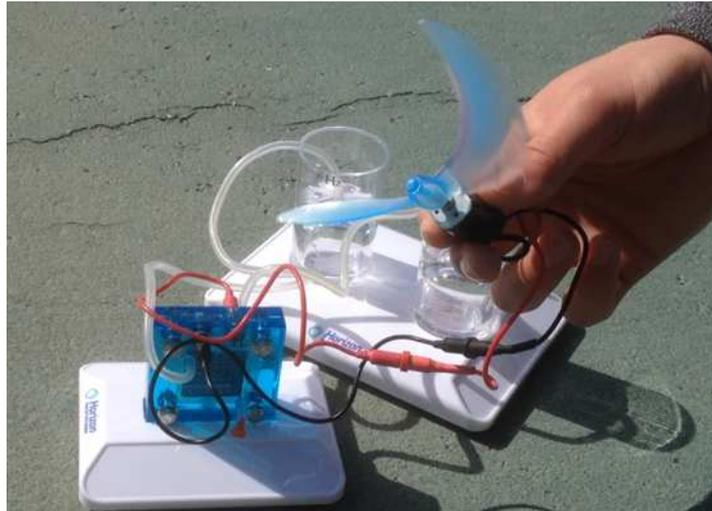
**Figure 3: Using Produced Hydrogen as Fuel for Functioning a Motor**
