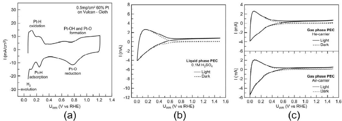
**Figure 5: Cyclic Voltammetry Curves on a Hybrid Fuel Cell Produced by the FOM Institute DIFFER**
