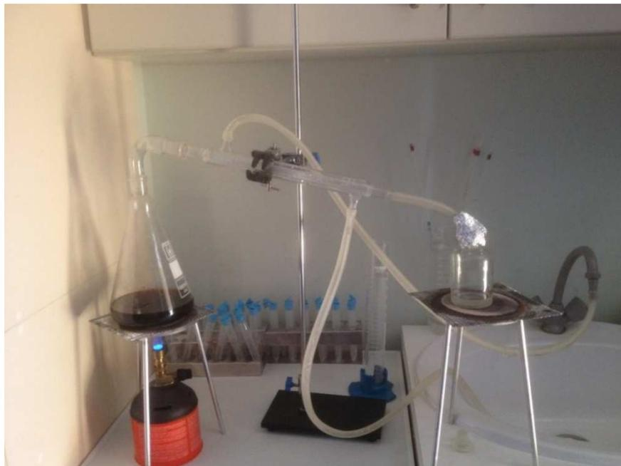
**Figure 4: Distillation of Contaminated Water**
